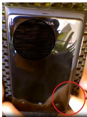
Figure 4: Camera button on the Windows Phone is confused with the power button.
