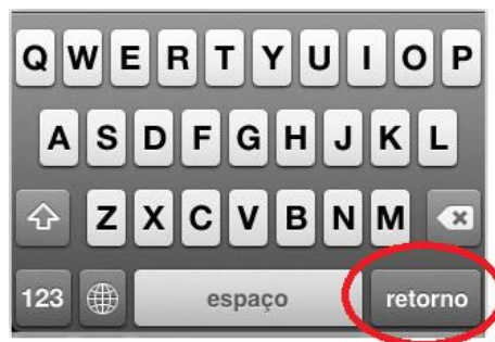
Figure 3: The word “return” or “retorno” confuses users into thinking they will return to an earlier screen or to an earlier operation on the iOS.
